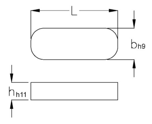
b = 8 h = 7 L = 16.0 Tolerance b = 0.036 Tolerance h = 0.090 Tolerance L = -0,2
